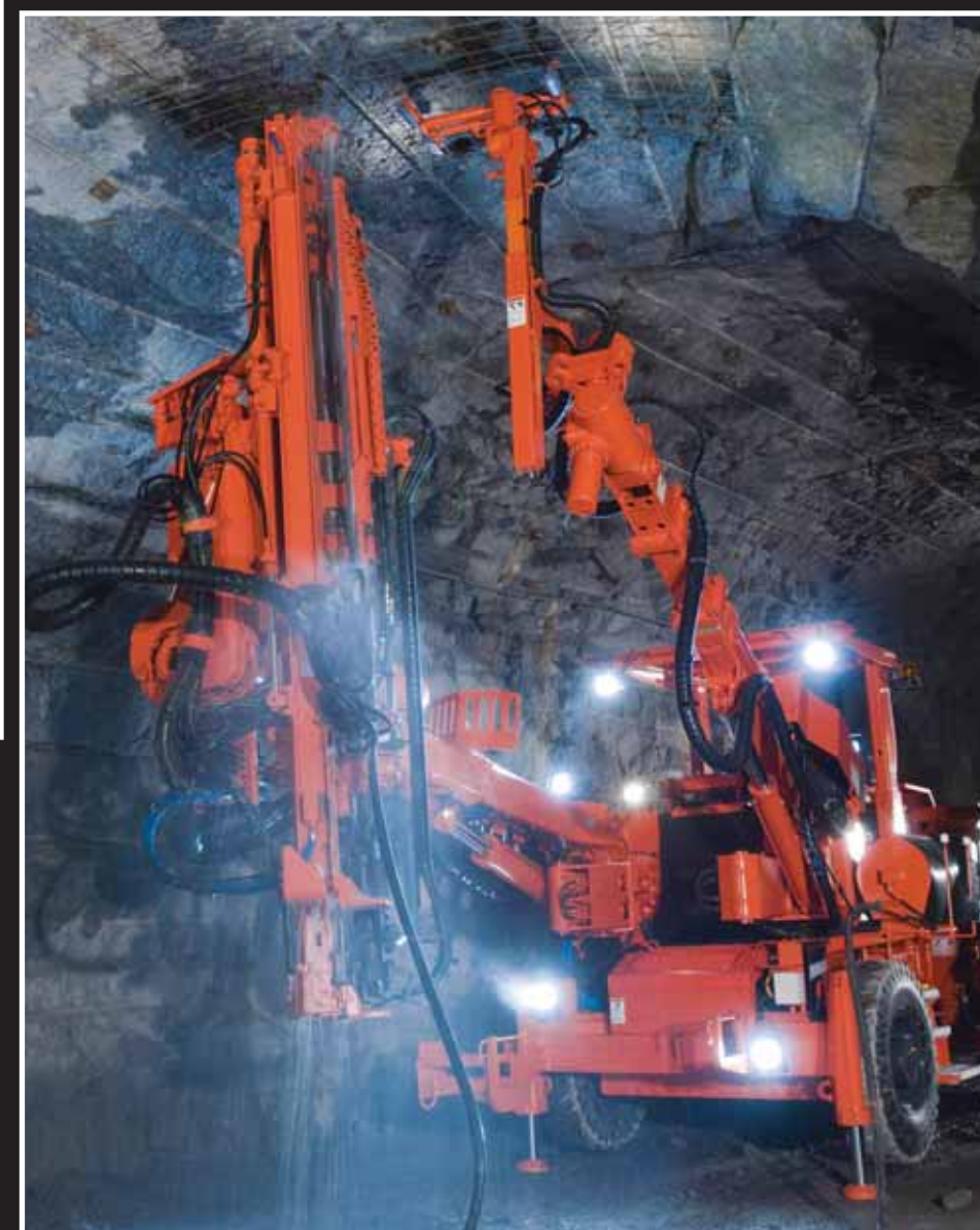
Top: A DL420 production drill, mounted on a TC7W articulated carrier, with a boom that allows a 360-degree rotation of the LF1500 drilling module.
